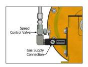
**Step 6:** Ensure the speed control valve is in the closed position, and connect the gas supply line. **A regulator is required if the supply gas pressure exceeds 35 psig.** *Note: BR5100HP and BR5100H models are equipped with a regulator (BA-1718) that can be used up to 220 psig. If required, a regulator (BB-0040A) for supply gas up to 5500 psig is available.* To prevent moisture or debris from entering the pump, a filter should be installed on the supply line.
