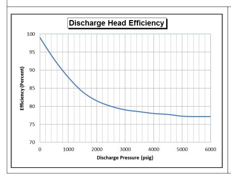
**NOTE:** With an increase in discharge pressure, the volumetric pumping efficiency of the pump head decreases as shown in the graph.
