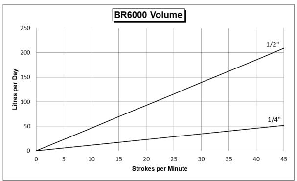
NOTE: Volumes based on 0 psig Discharge Pressure and Full (1") Stroke.
