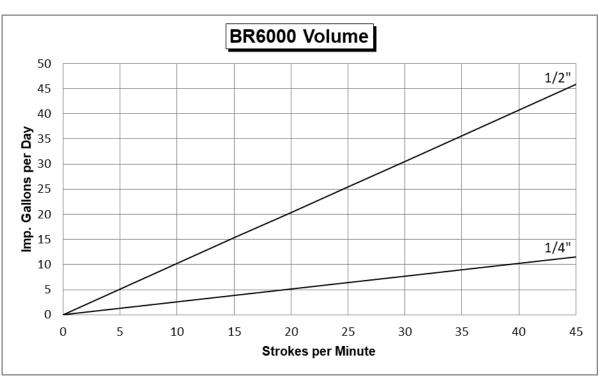
NOTE: Volumes based on 0 psig Discharge Pressure and Full (1") Stroke.
