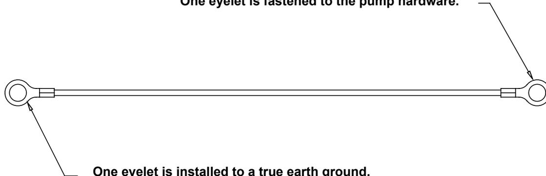
One eyelet is installed to a true earth ground.
