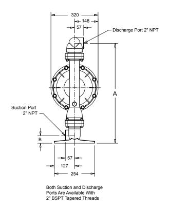
Note: The pump is be mounted in a horizontal position
