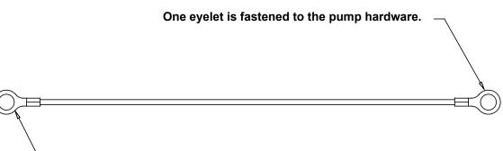
One eyelet is installed to a true earth ground. (Requires a
