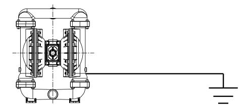
This 8 foot long (244 centimeters) Ground Strap (Item 38) is shipped with the eyelet end fastened to the pump hardware.
