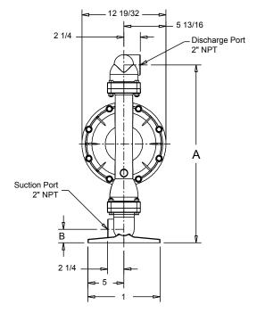
Both Suction and Discharge Ports are Available With 2" BSPT Tapered Threads
