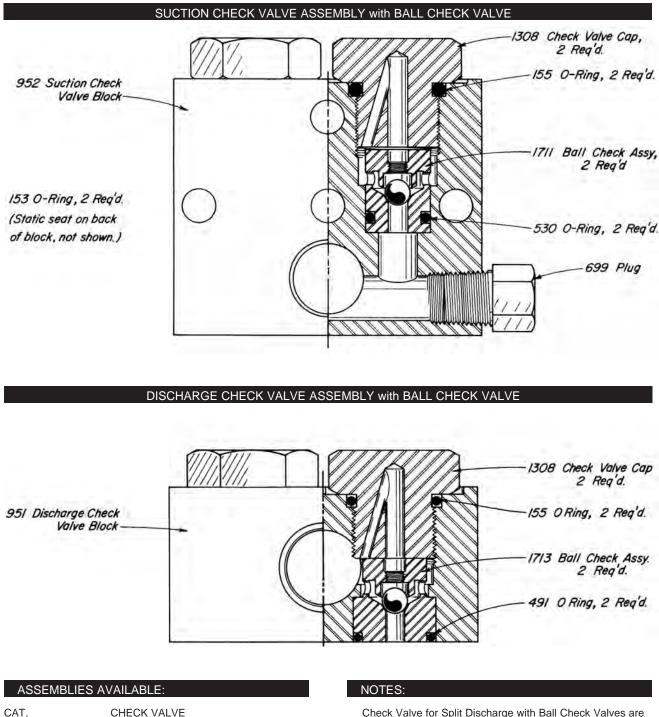
Check Valve for Split Discharge with Ball Check Valves are available.
