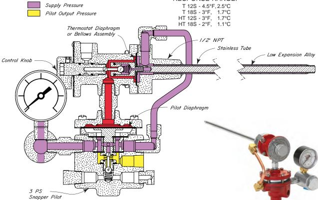
DIRECT SNAP THERMOSTAT DUCTILE IRON or STEEL
