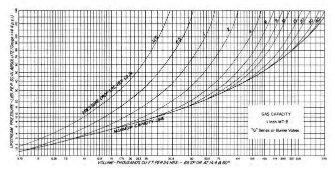
Gas capacities are based on pressure taken immediately upstream and downstream from the regulator in a wide open position.
